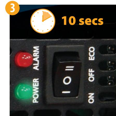
3. After 10 seconds, turn the toggle switch back to the 'ON' position.
