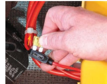
Remove the 20 amp fuse from the inline fuse holder on positive side of the 130 amp hour battery.
