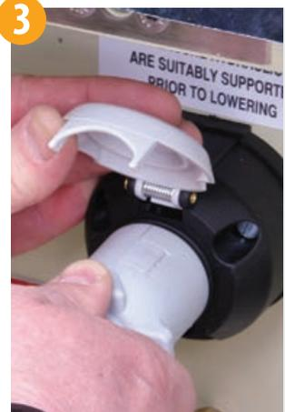
**Check wander lead/ hydraulic remote plug connection**
