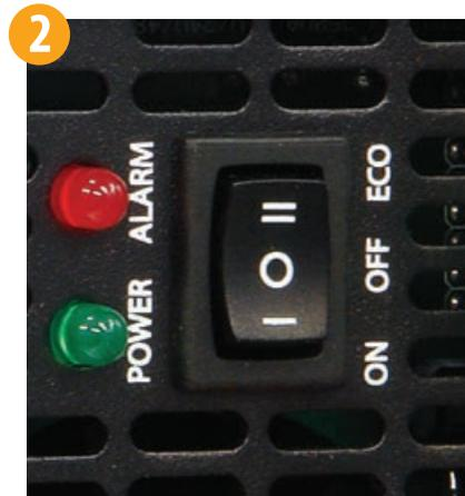
2. Turn toggle switch on inverter to the 'OFF' position.
