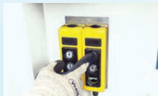
Push button controls to lower front and rear hydraulic rams
