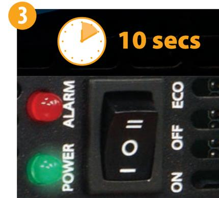
3. After 10 seconds, turn the toggle switch back to the 'ON' position.
