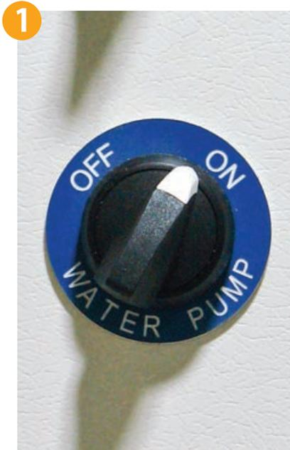
1 Check toggle switch in canteen area is in the 'ON' position.
