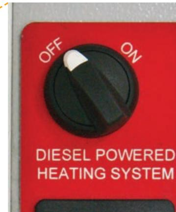
Turn the heater power isolator, situated on the 12V enclosure panel in the toilet area, anticlockwise to the "OFF" position.
