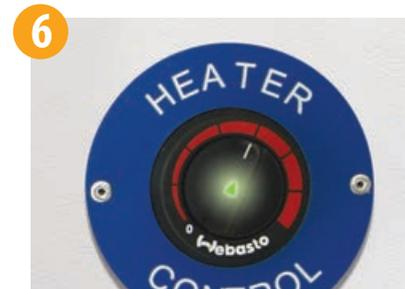
6 Finally, turn the heater control in the canteen clockwise to the "on" position; you should now see a solid green triangle in the centre of the heater control to show the heating is in working order.
