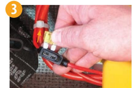
3 Remove the 20 amp fuse from the inline fuse holder on positive side of the 130 amp hour battery, positioned under seating in the drying area.
