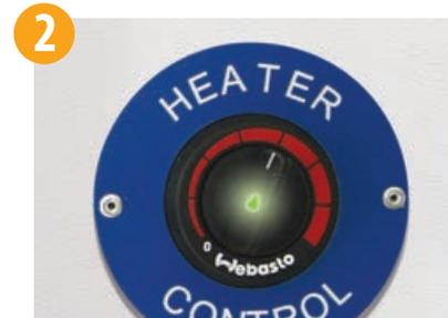
2 Turn the heater control clockwise to the "on" position, so that the error code is being given.
