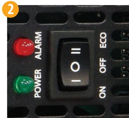
2. Turn toggle switch on inverter to the 'OFF' position.
